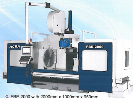
○ FBE-2000 with 2000mm x 1000mm x 950mm (1500mm) travel, 2100mm x 1050mm table
