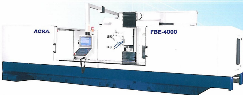
○ FBE-4000 with 4000mm x 1000mm x 950mm (1500mm) travel, 4100mm x 1050mm table
